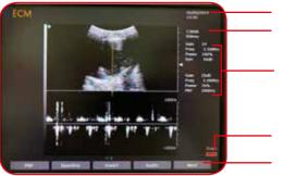
PRFSelect value.BaselineSelect the spectrum. The<br/>frequency/velocity is upda-<br/>ted on display.InvertInvert the frequency/velo-<br/>city scale. It is updated on<br/>display.AudioAudio output volume.FilterPW Wall Filter.PowerTransmit Power.
