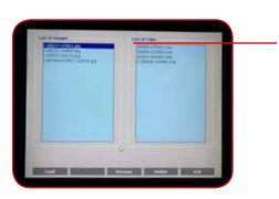
Review display includes the images and clips list. System will explore USB before exploring the internal memory. In order to access to internal memory, remove any connected USB device.
